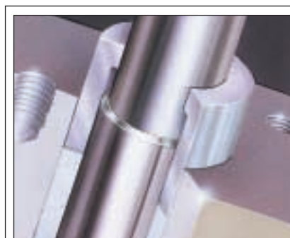
Blow-out proof stem design complies with API 609 criteria to guard against catastrophic leakage and stem blow-out in the event of shaft failure.
